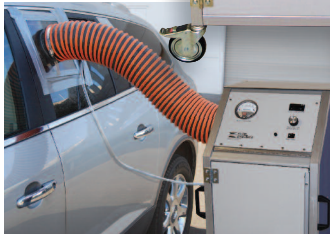
Body Leakage Tester in a test cell showing blower hose and pressure averaging wand inserted into rear window.
